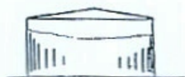
ORDINARY CONE ROOF TANK
